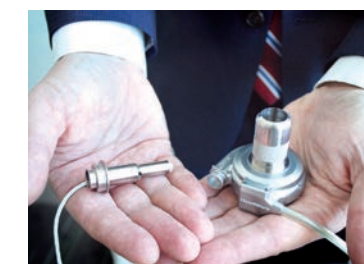
The pediatric VAD, roughly the size of an AA battery (left) vs. the size of an adult VAD.
